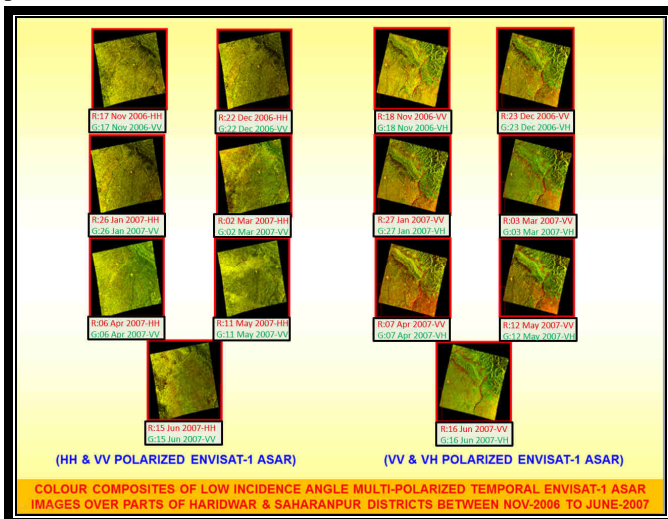
Fig-1: Color-composite of low incidence angle multi-polarized (HH/VV & VV/VH) ENVISAT-1 ASAR images over parts of Haridwar and Saharanpur districts between November-2006 to June-2007
